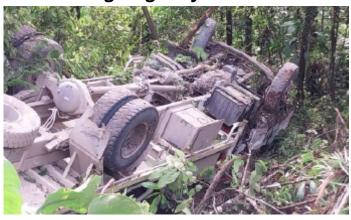
On the 18th of March 2024 at 15:46 the OTML F200 rolled over at KM 94 along a narrow pass on the Tabubil-Kiunga Highway. The truck involved was an Isuzu FVR truck modified as a tire truck with a Mobile Hiab attached to the back of the cabin, bearing the plate number DAC 501. The accident was caused by the driver's loss of concentration, driving error, and poor communication.
